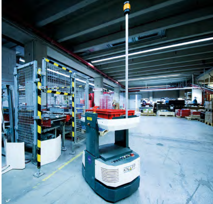
The autonomous mobile robots convey trays from the goods-in area to the infeed point of the conveyor system, from which the trays are transferred for storage into the OSR Shuttle™.
