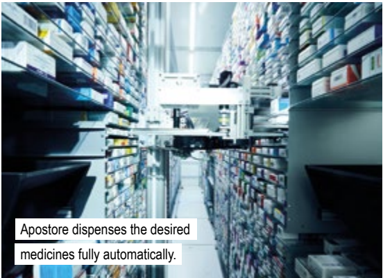
Feeder OCR makes it possible to fully automatically store medicines in the Apostore.
