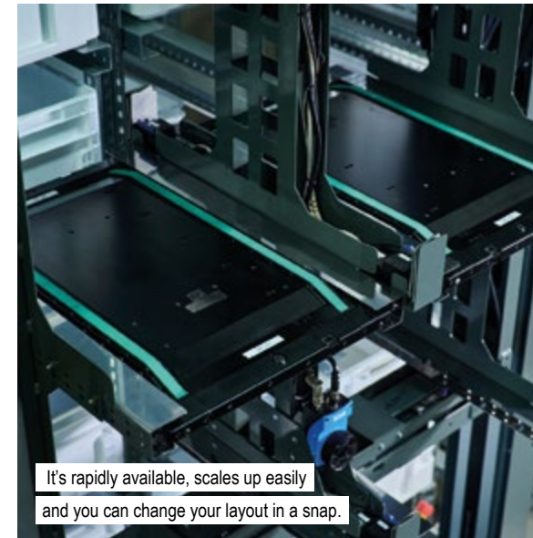
The AMRs travel with two robotic load-handling devices, called Sat Bots. These nimble little robots dash on and off the AMR to store and retrieve containers.
