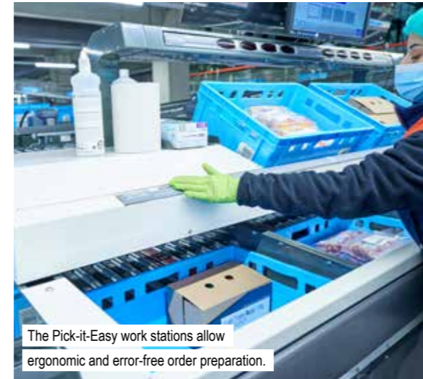
KiSoft Pick-to-Light guides the employee through the picking process.
